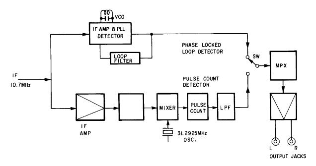
The phase locked loop has superior sensitivity and low noise characteristics, whereas the pulse count detector system excels with highest linearity and lowest THD operation. The PLL operates at low RF levels and the PCD is automatically switched in above 38 dBf, resulting in performance near theoretical limits.
