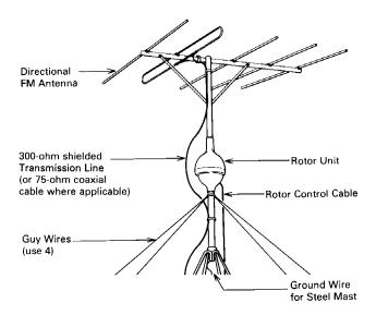
Another important factor is the type of lead-in wire to use. Unshielded lead-in wires, such as 300-ohm twin lead, can act as an omnidirectional antenna, and can cancel the directional benefits of your antenna. Therefore, we recommend using a balanced, shielded 300-ohm cable or a coaxial 75-ohm cable with a 300-to-75 ohm matching transformer at the antenna. These types of shielded cable effectively prevent the lead-in from contributing to multipath distortion.
